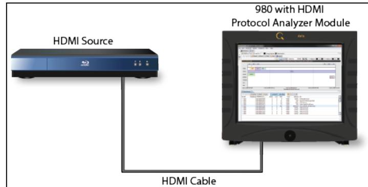
**Figure 3: Configuration #1: 980 Direct Capture**
