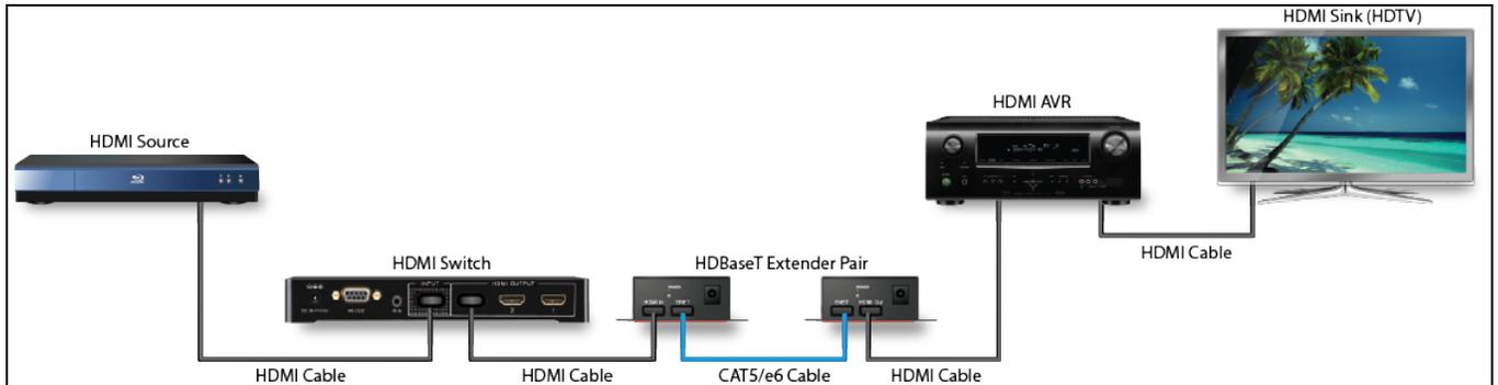
**Figure 1: Typical HDMI distribution network with HDBaseT extender**
