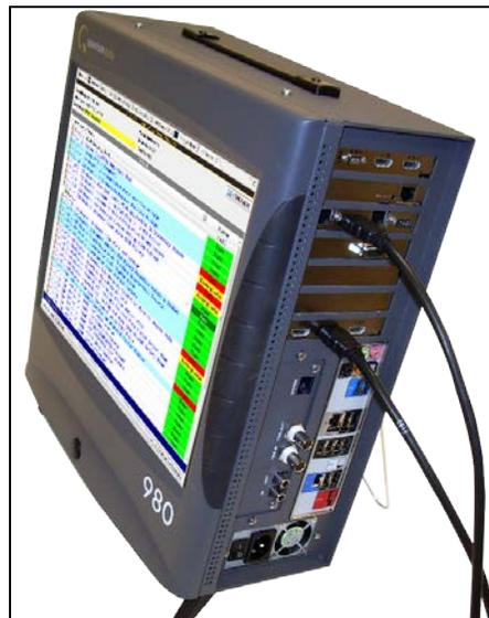
**Figure 2: Quantum Data 980B with Protocol Analyzer Module
