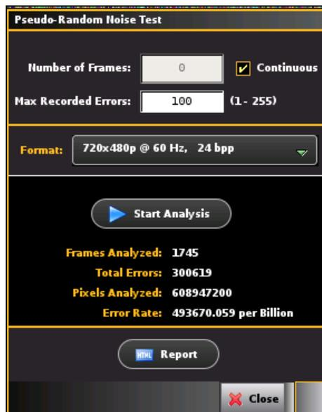
Figure 11: Screen shot of real time pixel error counts on PRN test
