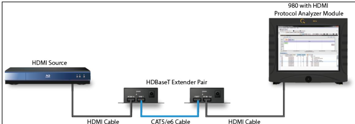
**Figure 4: Configuration #2: 980 Capture through HDBaseT Extender**
