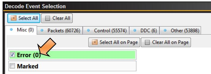
Figure 8: Screen shot of captured (BCH) error counts
