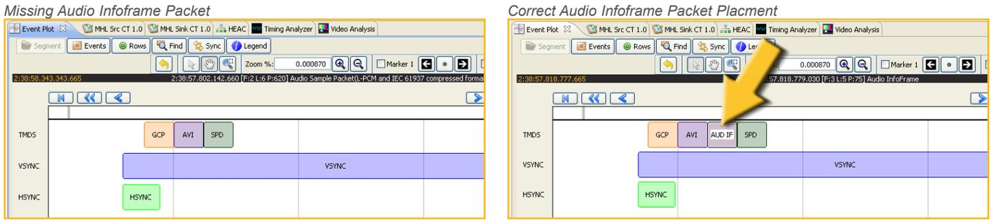
In other cases, audio dropout can occur when the transmitter sends audio packets in a cadence that the receiver chip cannot accept. The 980 enables you to examine the precise placement of the audio packets in the blanking intervals. You can zoom in and out and pan across the capture data to examine the arrangement of audio packets in the blanking in proximity to the occurrence of the audio dropout (Figure 5).
