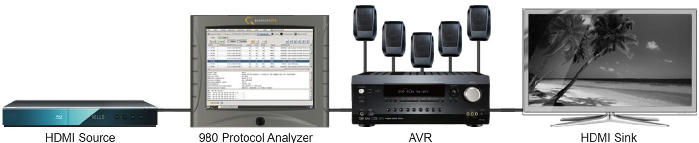
Part of the configuration of the capture criteria is ensuring that you capture enough of the important types of data. The manual capture is used so that you can monitor the downstream audio rendering device. When using the manual capture it is important to set the capture trigger buffer properly so that you capture the data when the audio dropout occurs (Figure 3). To do this you configure the capture trigger position buffer to the right most side using the sidebar.
