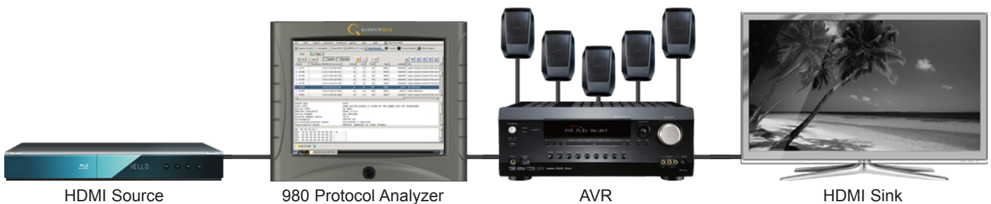
Figure 2: Basic Setup for Monitoring Encrypted and Unencrypted Audio Related Data.
