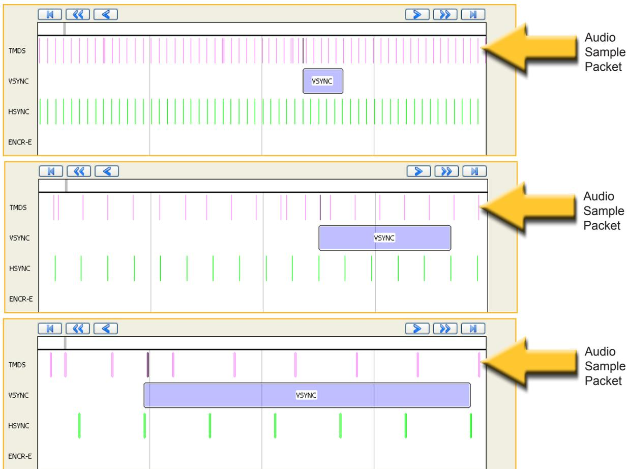
These are just a couple of the primary causes of audio dropout. Because the 980 Protocol Analyzer can capture all audio related packets between a source and sink and assign precise timestamps, other causes of audio dropout can be isolated as well.
